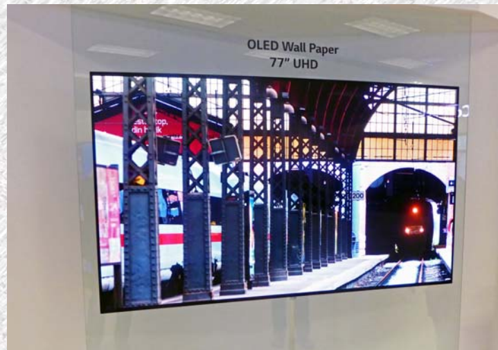
LG 77-INCH 4K (3840x2160) OLED TV, MEASURING 6MM THICK
